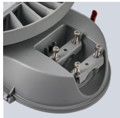
Specialist four bolt pole mounting mechanism allows fixing to Ø42mm to Ø60mm poles with a 5° adjustable angle.
